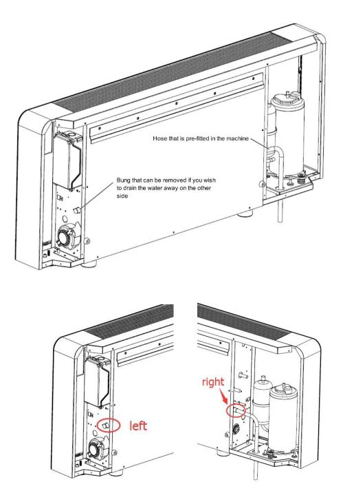
Connect the condensate hose (16mm diameter) and ensure that the water is flowing downhill with no kinks or blockages. You have the choice of fitting the drain on the right or left side. The hose on the right is pre-fitted, if you wish to change to the left, remove the bung from the left and swap it with the hose on the right.
