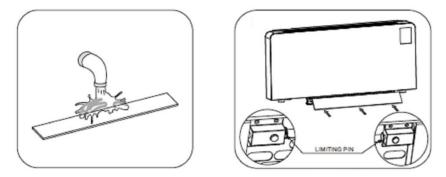
Wash the filter in water and allow to dry fully before refitting. Once the filter is dry reinsert and allow the safety springs to clip back into place on the right and left.
